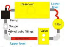
pump was above **Figure 5: Hydraulic layout** the motor. Due to
